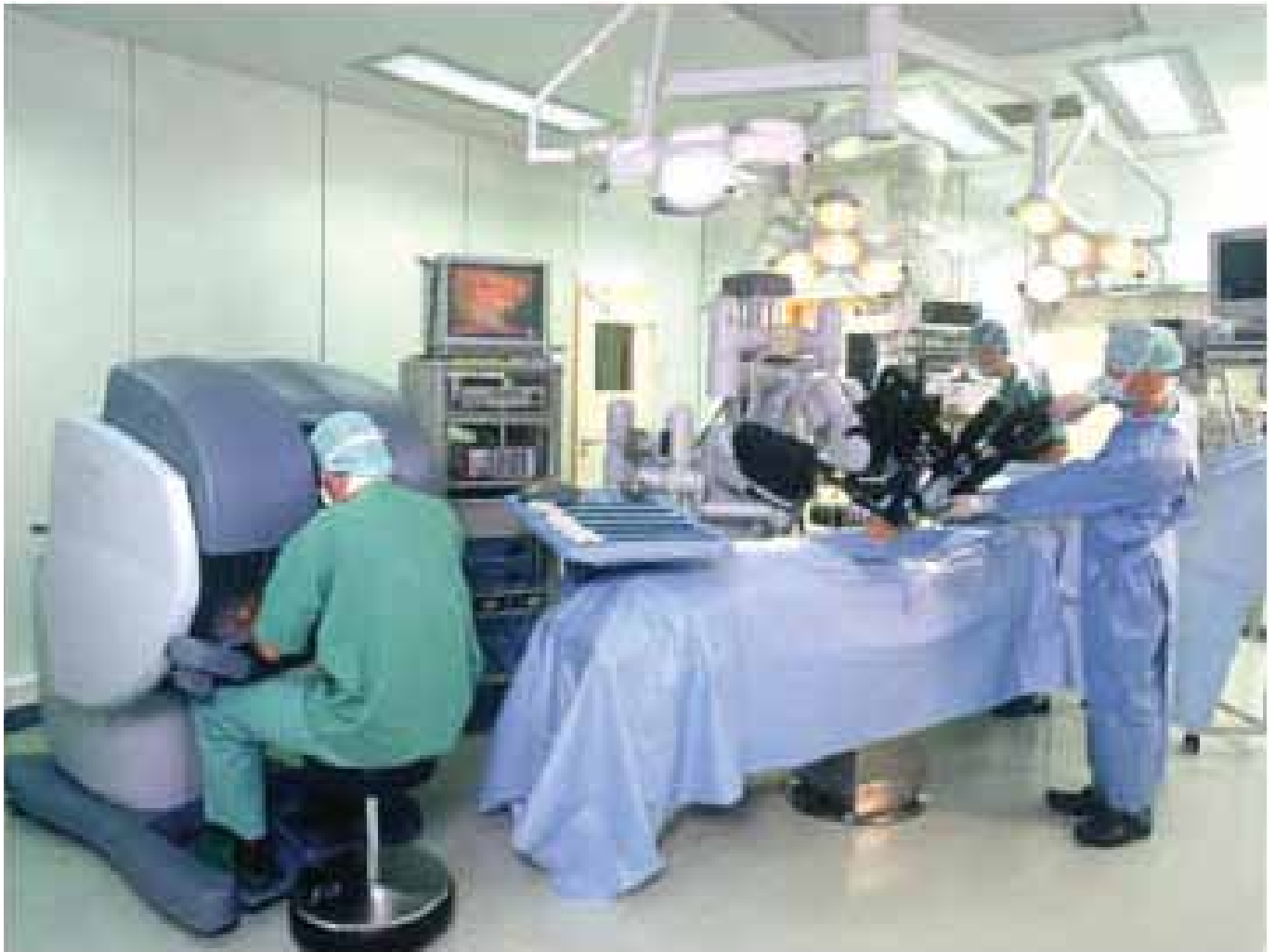
In the da Vinci system, the surgeon sits at a viewfinder (left) and remotely manipulates probes and instruments on actuator arms over the operating table.
