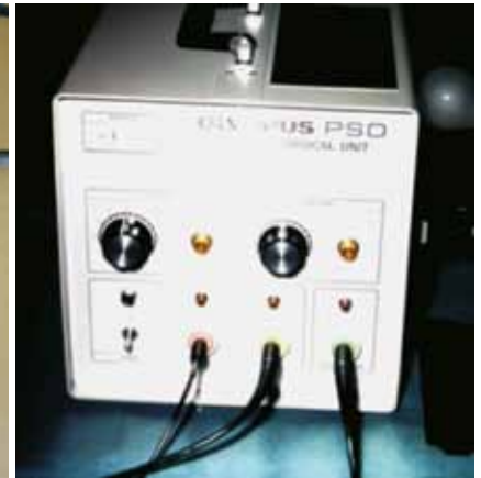
Fig 36-2c. Diathermy apparatus with special safety device for use in endoscopy. The light bulb was being tested before each endoscopy. Photo Arne R Rosseland SiA 1975
